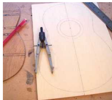
STEP 1. The soundboard dimensions and rosette marked out
